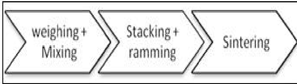
Figure 1.2 Powder Metallurgy Process
